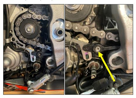
6. Assembly shift shaft support and sprocket cover, using the following screws lenght:
