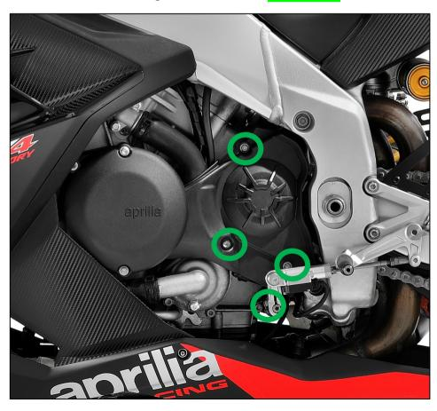
2. Remove the plastic cover; apply a mark between shift leverage and shaft and disassemble leverage:
