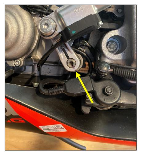
3. Remove the following 2 OEM threaded bushes with 12 mm wrench:
